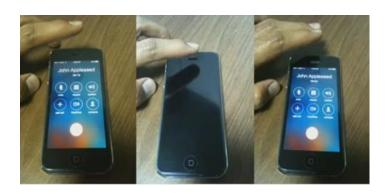
In present Android devices, the proximity sensor triggers as the user's face is close to the screen, switching off the screen and preventing any errant soft-button presses by the skin as well as saving battery power.
